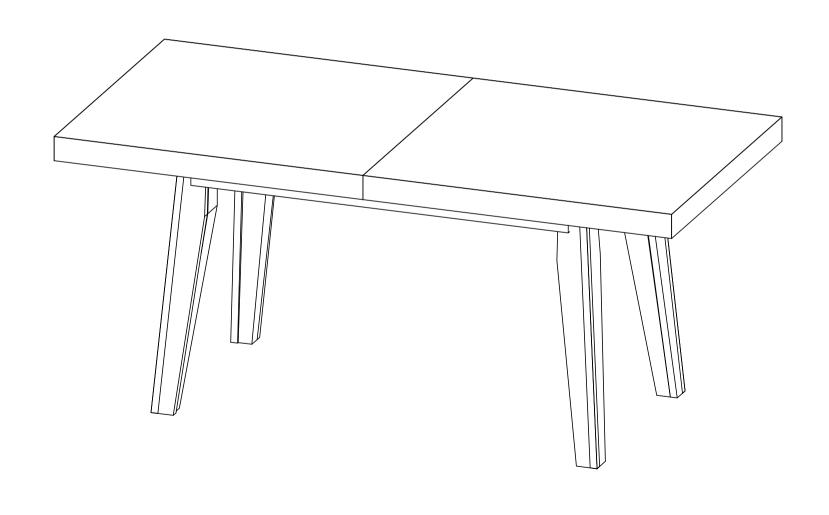
Put PART-A and PART-B together tightly. Use L-Wrench No.5 to drill in JCB M8x40 into the drill holes.
