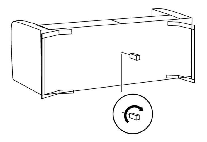
please find the fixing hole underneath, place the adjustable plastic leg
